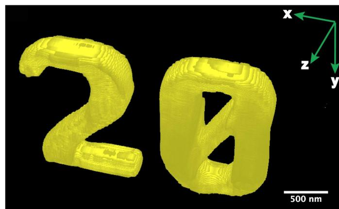
Figure 4. Reconstructed 3D ptychographic image of “20” on an Au test pattern. A total of 31 projections were obtained with 4° rotation step. Each projection was acquired by performing a fly scan, then reconstructed using ePIE with five probe modes [22].
