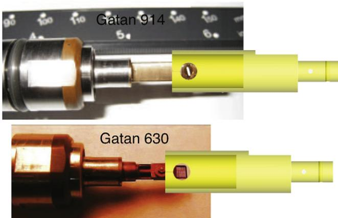
**Fig. 1.** Gatan 914 cryo-sample holder uses 3 mm diameter round grids, and Gatan 630 holder uses rectangular grids with a width of 3 mm. The anti-contaminator coaxially fits both holders. There are two holes on its side wall, which allow the X-ray beam to illuminate the sample grid and the diffraction signal to propagate without being obstructed.
