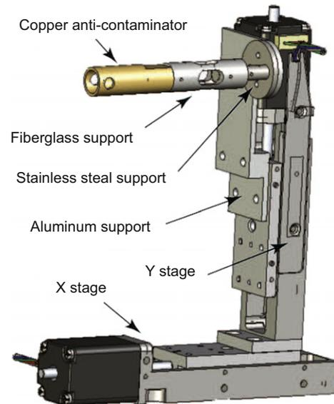
**Fig. 2.** The anti-contaminator is a hollow copper rod coated with gold. It is mounted on a Micos VT-21 stepper motor stage. The ACD is thermally isolated from the warm stage by a hollow fiberglass support and a stainless steel support.
