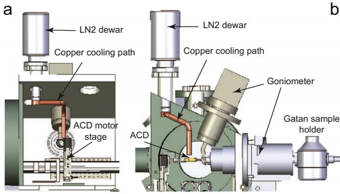
**Fig. 3.** The anti-contaminator is cooled by a liquid nitrogen dewar, which is mounted on the top of the microscope chamber. A copper rod attached to the dewar bottom is bent to fit the chamber and extends to about 1.27 cm away from the anti-contaminator. The tail of the copper rod is connected to the ACD by a 5 cm long, 1.27 cm wide copper braid (not shown in the figure). (a) The side view of the chamber with cooling path. (b) The cross-section view along X-ray direction.
