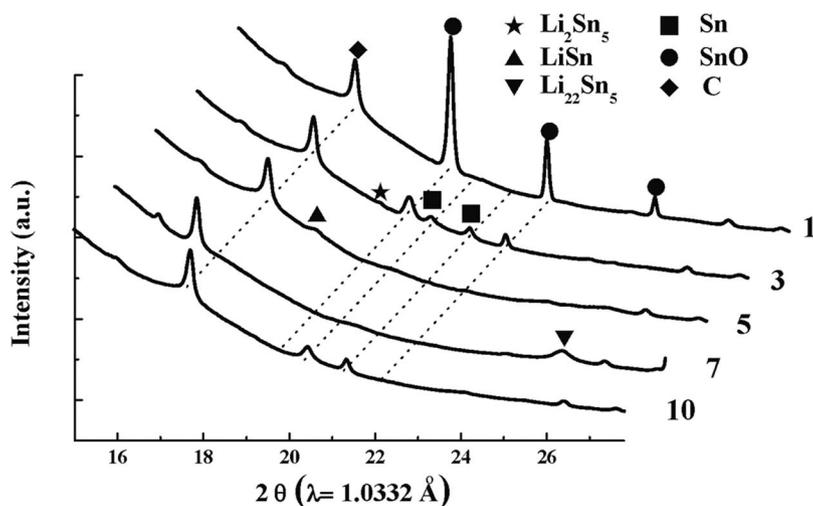
**Figure 4.** Synchrotron X-ray diffraction data of the SnO electrode acquired during the first lithiation/de-lithiation cycle. The numbers shown to the right end of the curves are same as indicated in Fig. 3.
