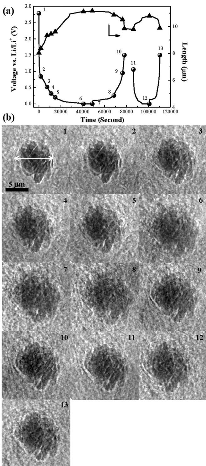
**Figure 3.** (a) Voltage-vs.-time plot of the SnO electrode and particle dimension-vs.-time plot of the SnO particle shown in (b) during the first two lithiation-delithiation cycles; (b) the snapshots of a selected particle during the same period. The points and numbers shown in (a) mark the moments at which the snapshots of corresponding numbers in (b) have been taken. The arrow in the panel #1 in (b) indicates the direction along which the particle dimensions have been measured.
