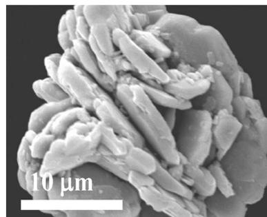
Figure 2. SEM micrograph of the tested SnO particle.
