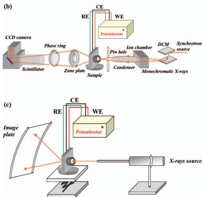
Figure 1. Schematic illustration of (a) the coin-cell assembly for in-situ synchrotron studies; (b) in-situ transmission X-ray microscopy; and (c) in-situ X-ray diffraction. The working electrode in (a) is a free-standing film containing SnO particles embedded within a graphite matrix.
