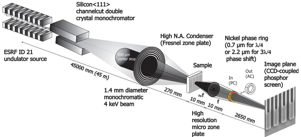
**Figure 1.** Schematic of the x-ray microscope (TXM) in Zernike phase contrast mode installed at ID21 at the European synchrotron radiation facility (ESRF). In the ray diagram, only the radiation passing directly through the sample is shown, diffracted light is omitted for simplicity.
