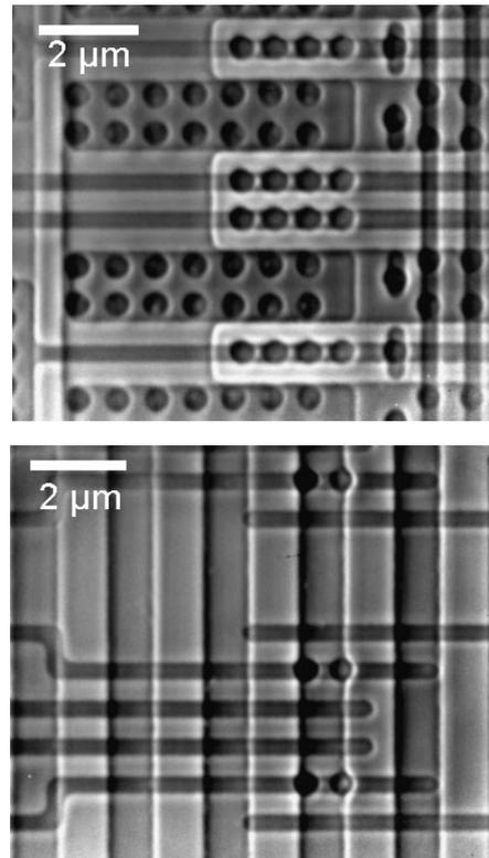
**Figure 4.** Copper interconnect structures, imaged with the ID21 transmission x-ray microscope in negative phase contrast, i.e. the direct, undiffracted light passing through the sample was phase shifted by  $270^\circ$  using a  $2.2\ \mu\text{m}$  thick nickel phase ring.
