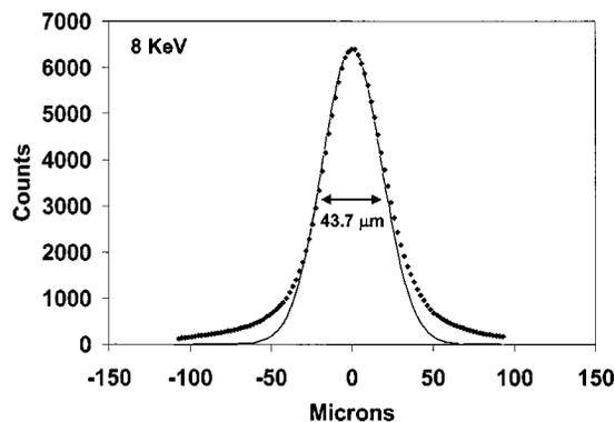
FIG. 5. Vertical profile of the 8.0 keV x-ray spot indicating the  $43.7\ \mu\text{m}$  vertical FWHM produced by parabolic Li CRL at the image plane. The data are fitted with a solid line Gaussian distribution of  $18.6\ \mu\text{m}$  standard deviation and  $43.7\ \mu\text{m}$  FWHM about its mean, which is the center axis of the Li CRL.
