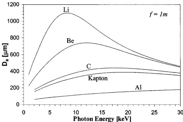
FIG. 2. CRL attenuation apertures as a function of photon energy for lenses with focal length of 1 m made of Li, Be, kapton, C, and Al. The figure establishes that x-ray CRLs assembled with Li unit lenses have about a factor of two larger apertures at the softer x-ray energy range of the figure (about less than 15 keV).
