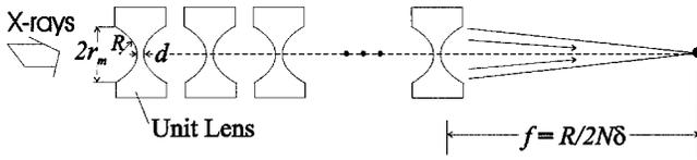
FIG. 1. X-ray focusing using compound refractive lens (CRL) comprised of a stack of  $N$  biconcave, parabolic unit lenses with on-axis radius of curvature  $R$ , minimum thickness  $d$ , and physical aperture diameter  $2r_m$  fabricated from 0.020-in.-thick lithium foil. The individual lithium unit lenses has a focal length  $f=R/2\delta$ ; however, the CRL has  $N$ -fold shorter focal length  $f=R/2N\delta$ .
