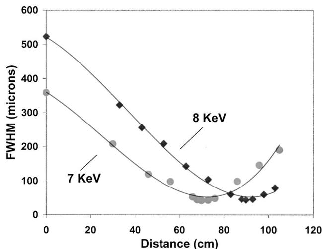
FIG. 4. Vertical profiles of 7.0 and 8.0 keV x rays focusing along the propagation direction. The minimum vertical FWHM of the image spots are  $41.6$  and  $43.7\ \mu\text{m}$  at 70 and 90 cm, respectively, for the respective 7 and 8 keV photon energies.
