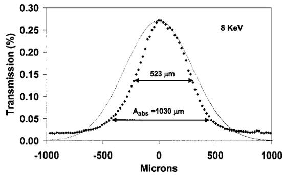
FIG. 6. Measured transmission through the CRL as a function of the radius of the lens. The figure shows the 1030  $\mu\text{m}$  attenuation diameter of the lens as well as the 523  $\mu\text{m}$  FWHM of the lens aperture. The solid line is the calculated transmission profile with an attenuation diameter of 1200  $\mu\text{m}$ .
