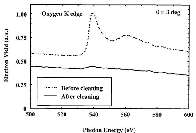
Fig. 3. Electron yield measurements (arbitrary units) on a Si(100) wafer at  $\theta = 3^\circ$  (grazing angle), performed at the ALS beamline 6.3.2; before cleaning (dotted curve) there is a pronounced peak at the O  $K$  edge (543.1 eV) that is due to the presence of the  $\text{SiO}_2$  on the surface; the peak becomes barely visible after surface cleaning (solid curve).
