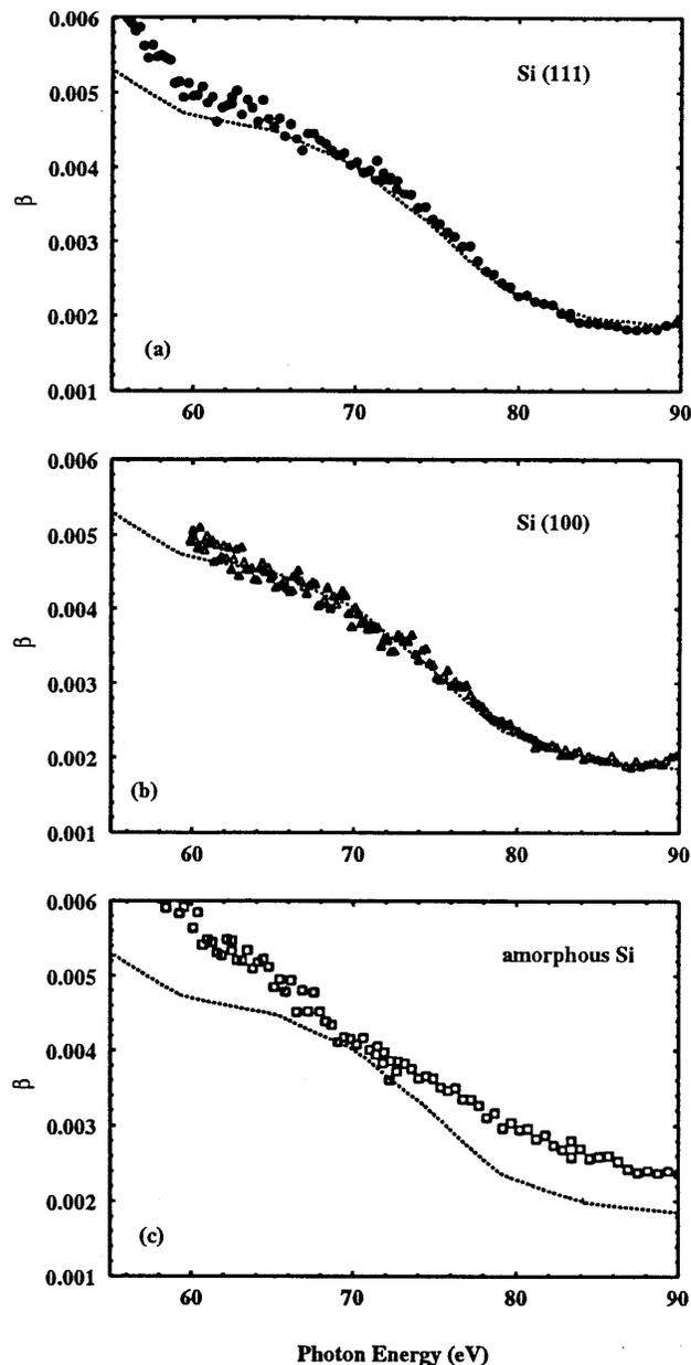
Fig. 8. Fitted values of  $\beta$  determined from reflectance measurements at the laser plasma source for (a) a Si(111) sample, (b) a Si(100) sample, and (c) an amorphous Si sample. Small corrections ( $\leq 10\%$ ) for the presence of residual contamination were applied for each of the sets of data. The dotted curves represent transmission data for Si(111) presented by Gullikson *et al.* in Ref. 4.
