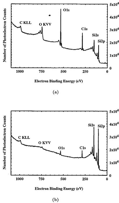
Fig. 2. XPS survey scan results for a Si(111) wafer (a) as received and (b) after H passivation.
