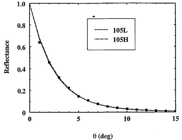
Fig. 6. Reflectivity curves calculated for  $s$ -polarized light and with  $\delta = -0.00725$ ,  $\beta = 0.0105$ , shown as point 105H in Fig. 5 and with  $\delta = -0.015$ ,  $\beta = 0.001$ , shown as point 105L in Fig. 5. The reflectance data at 105 eV for a Si(100) sample measured at the ALS beamline 6.3.2 are also shown.
