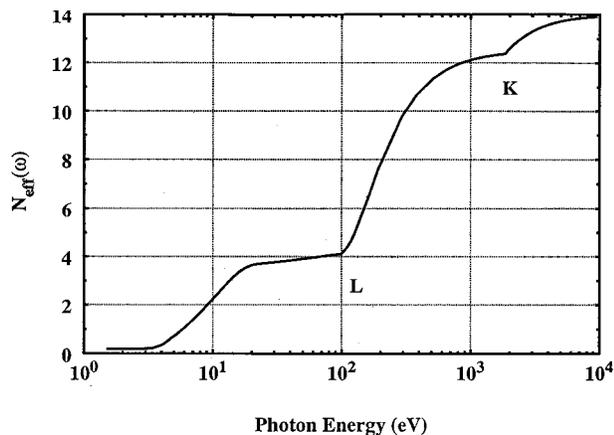
Fig. 1. Calculation of the left-hand side of the partial sum rule, Eq. (6), with the data for  $f_2$  from Ref. 1. Although Eq. (6) requires that  $N_{\text{eff}}(\hbar\omega \rightarrow 0) = 0$ , the calculation with experimental data gives  $N_{\text{eff}}(\hbar\omega \rightarrow 0) = 0.2$ . This missing oscillator strength should cause overestimation of  $\delta$  at low energies.
