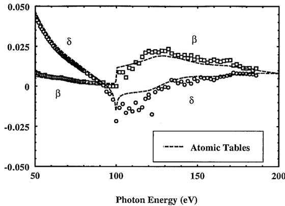
Fig. 4. Optical constants  $\delta$  ( $\circ$ ) and  $\beta$  ( $\square$ ) for a Si(100) sample measured at the ALS beamline 6.3.2. The values for  $\delta$  and  $\beta$  (dashed curve) from the atomic tables<sup>1</sup> are also shown.
