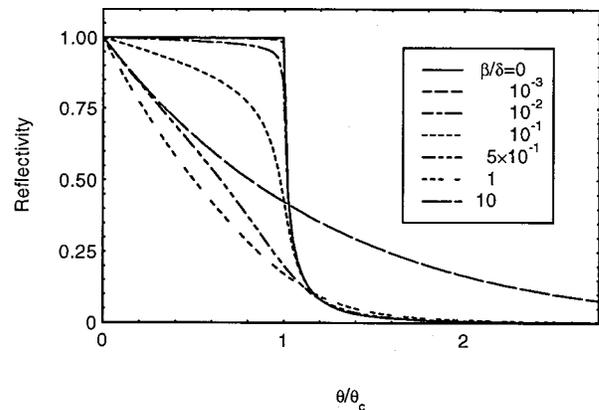
Fig. 7. Calculated reflectivity curves for  $s$ -polarized radiation and a range of  $\beta/\delta$  values. On the horizontal axis the grazing angle  $(\theta)$  is normalized to the critical angle  $\theta_c = \sqrt{2\delta}$ .
